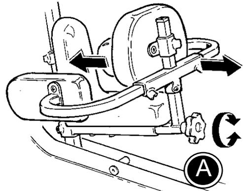
**!** When both head support and side supports are needed, the side supports have to be mounted on the body support bar. Please notice that Pony size 2+3 can not be equipped with both head support and side supports.
