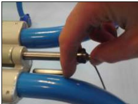
The locking pin is captured with the use of a tie so it can not be lost / misplaced. The rollator must not be used if this locking pin is missing. Contact Kingkraft immediately.
