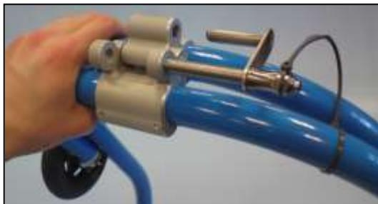
Whilst pushing the locking pin in, ensure the other smaller fixed pin locates into the smaller single hole in the clamp part around the main frame.
